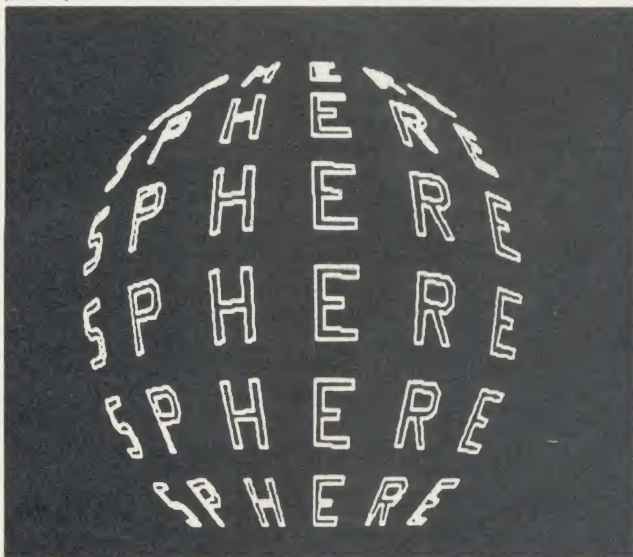
Figure 7. Mapping onto a spherical surface. The procedure that implements this is given in listing 6
